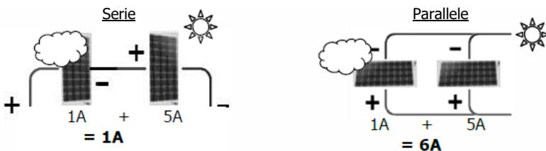
In case of parallel coupling, the panel power adds up.
