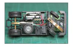
Finally, the model may be reassembled and improved with a few other details. For additional camouflage, the technical components may also be painted in the same paint as the frame so that the modification is not as noticeable.
